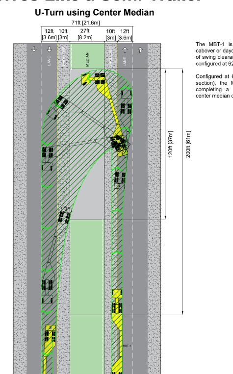
The MBT-1 is commonly used with a cabover or daycab tractor with 60in [1.5m] of swing clearance. The MBT-1 is usually configured at 62ft to 82ft [18.9m to 25m].
